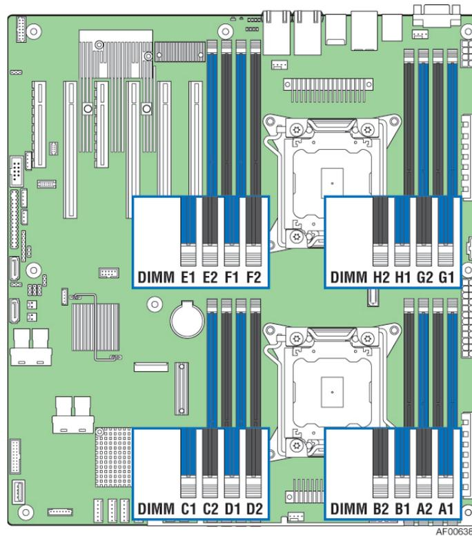
Figure 15. Intel® Server Board S2600CW DIMM Slot Layout
