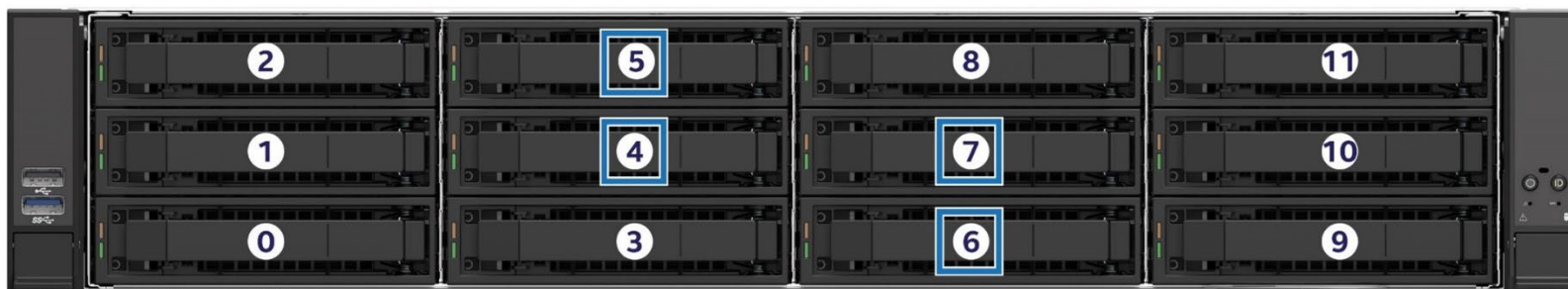
Figure 27. 2U 12 x 3.5" M50FCP2UR312 Front Drive Bay Configuration
