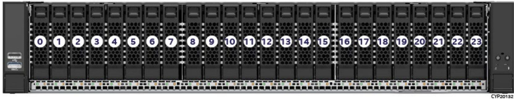
Figure 25. 2U 24 x 2.5" M50FCP2UR208 Front Drive Bay Configuration
