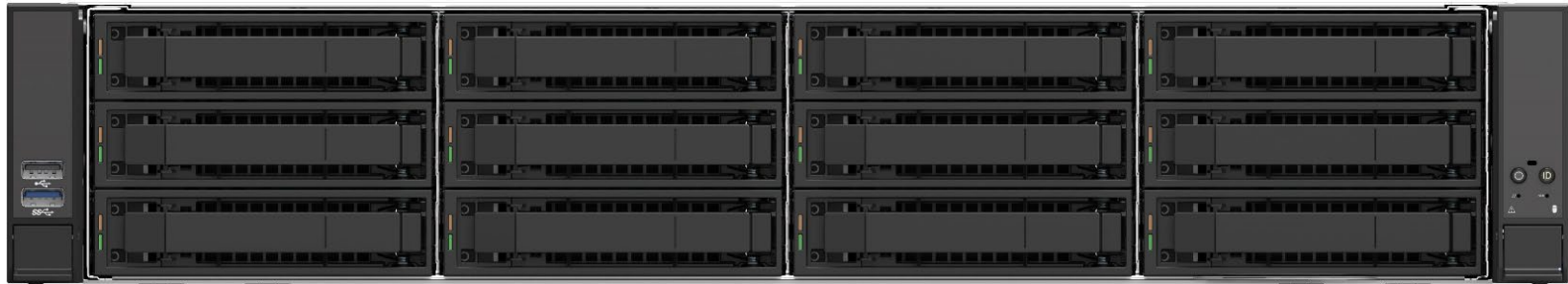
Figure 12. 2U 12 x 3.5" Front Drive Bay Configuration – iPC M50FCP2UR312
