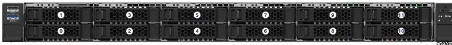
Figure 22. 12 x 2.5" Front Drive Bay Configuration – M50FCP1UR212
