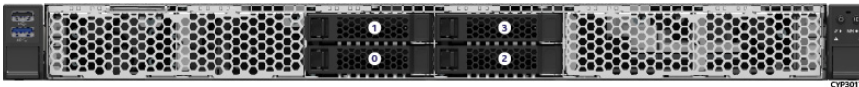
Figure 21. 4 x 2.5" Front Drive Bay Configuration – M50FCP1UR204
