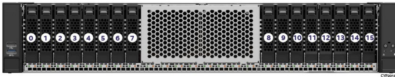
Figure 24. 2U 16 x 2.5" Front Drive Bay Configuration
