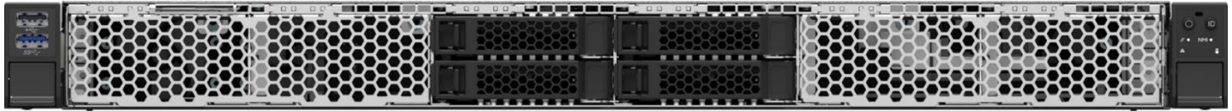
Figure 5. 4 x 2.5" Front Drive Bay Configuration – iPC M50FCP1UR204
