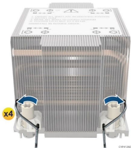
Figure 93. Processor Heat Sink Anti-tilt Wires in the Outward Position
