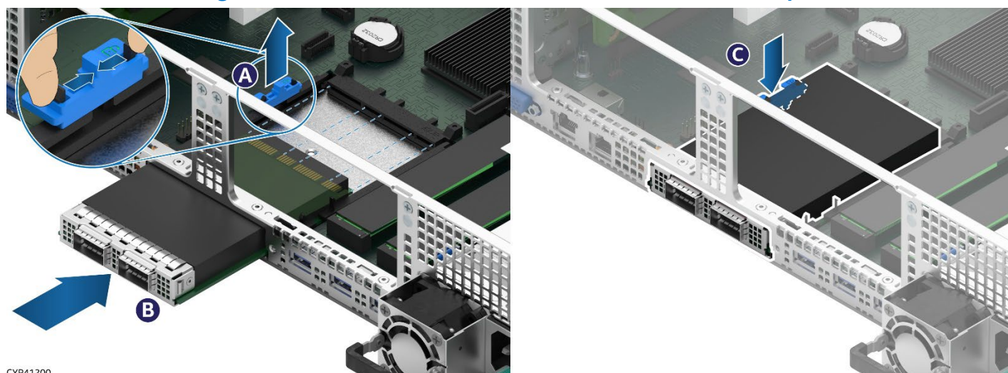
Figure 61. OCP 3.0 Add-in Card Installation – Internal Lock Option
