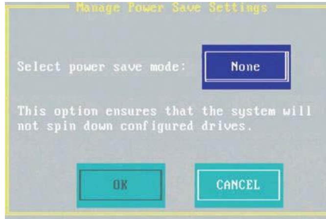
Figure 63. RCU – manage drive group power save settings
