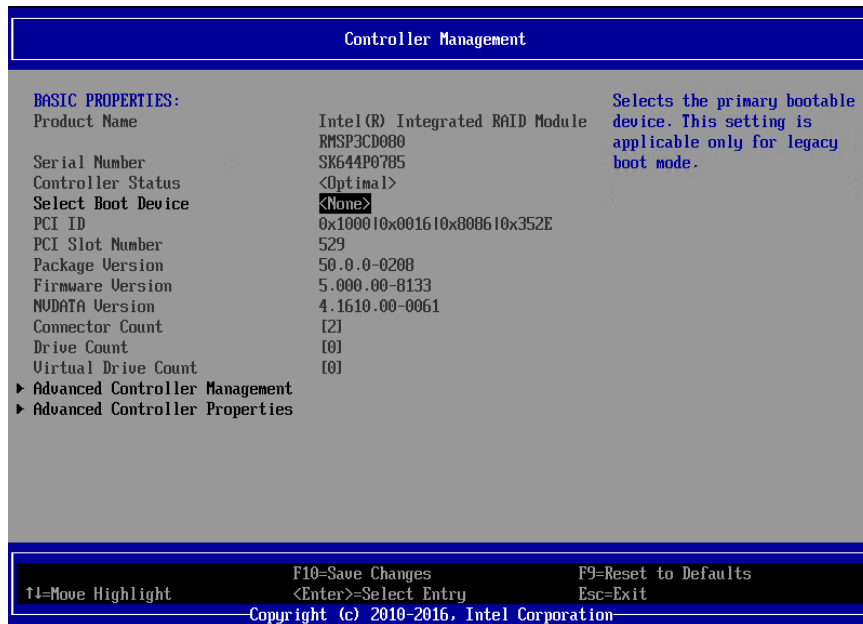
Figure 78. HII CU - Controller Management Screen
