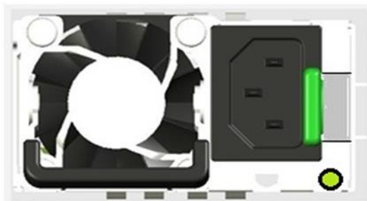
AC Power Cable Connectors
