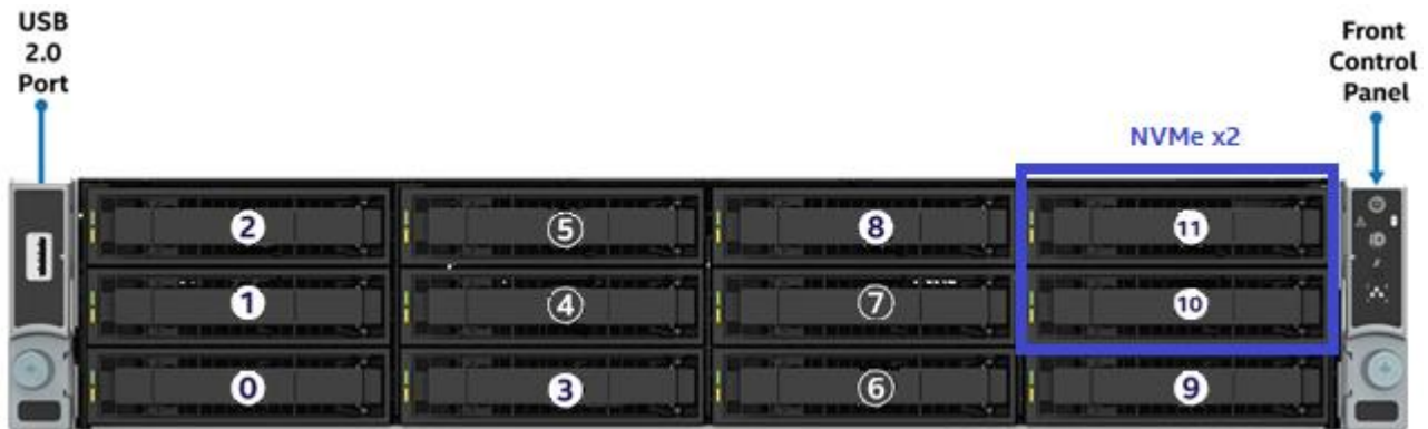
Figure 44. 3.5” drive bay, 12-drive configuration
