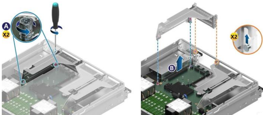
Figure 13. Intel® Storage Adapter Card Installation (Riser Card Assembly Removal)
