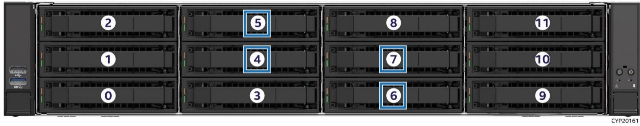
Figure 77. 12 x 3.5" Front Bay Drive Configuration – M50FCP2UR312
