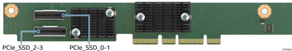
Figure 81. PCIe* NVMe* Riser Card for Riser Slot #3
