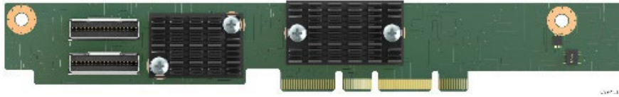
Figure 54. PCIe NVMe Riser Card for Riser Slot#3
