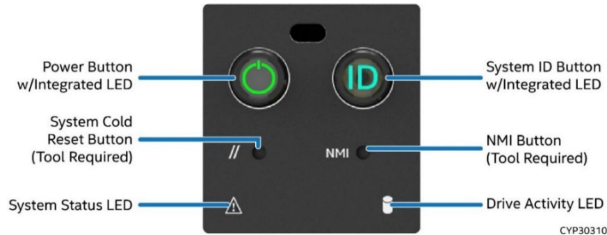
Figure 93. Front Control Panel Features
