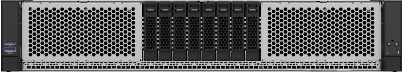
Figure 8. 8 x 2.5" Front Drive Bay Configuration – M50FCP2UR208
