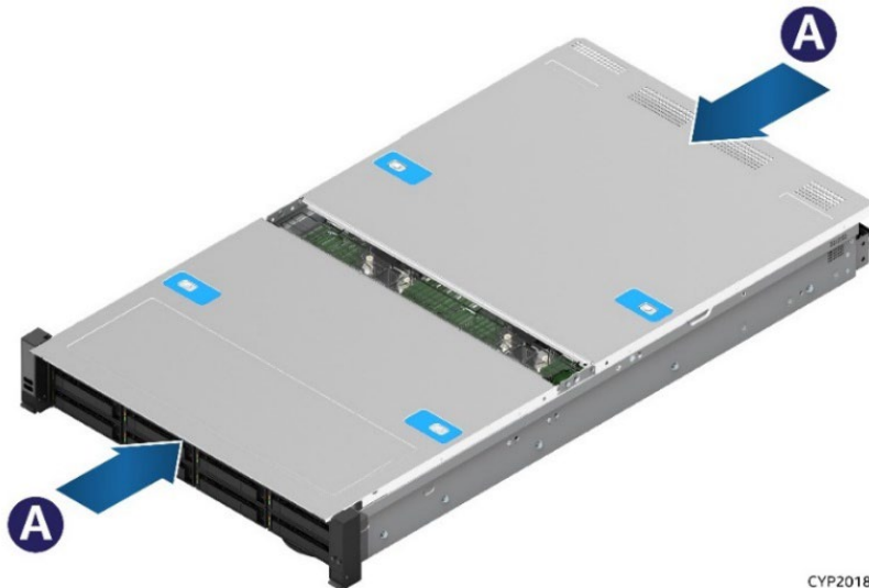
Figure 25. System Top Cover Installation
