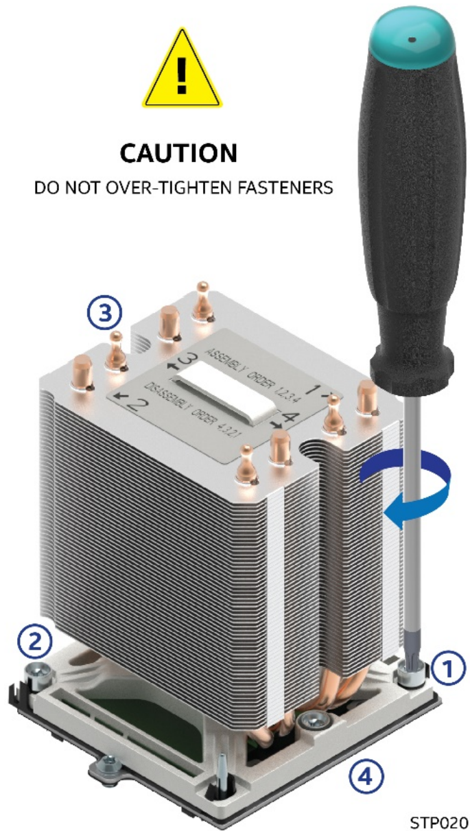
Figure 19. Tightening the heat sink screws
