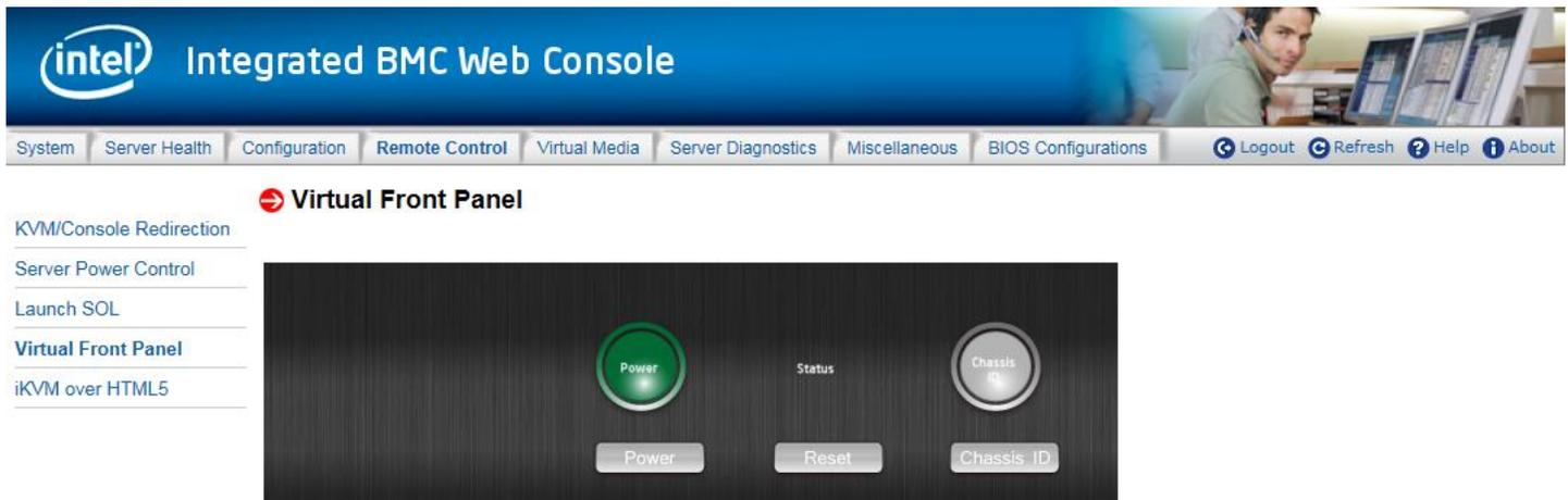
Figure 78. Remote Control Virtual Front Panel Page
