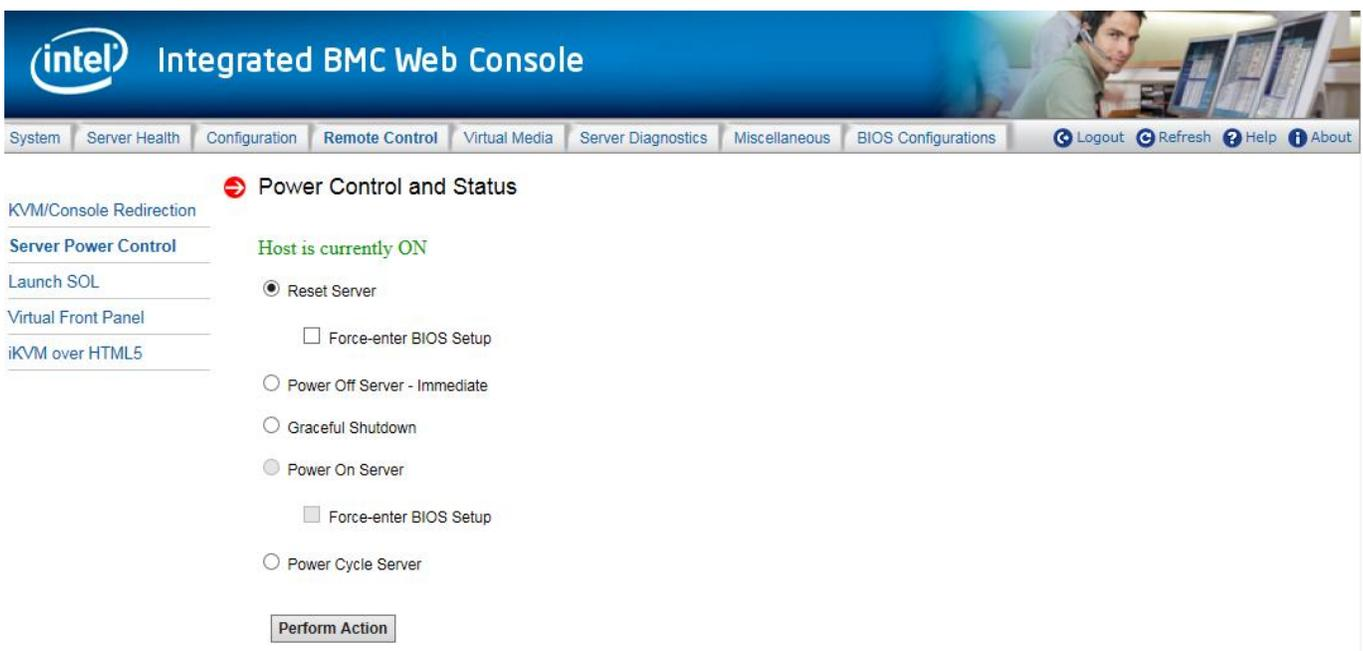
**Figure 75. Remote Control Server Power Control Page**
