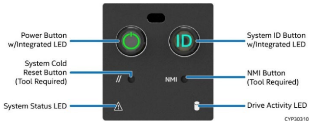
Front Control Panel
