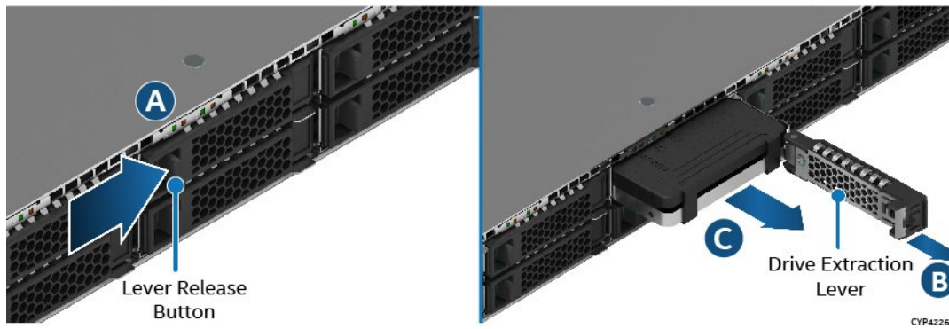
Figure 51. Drive Removal from Drive Bay
