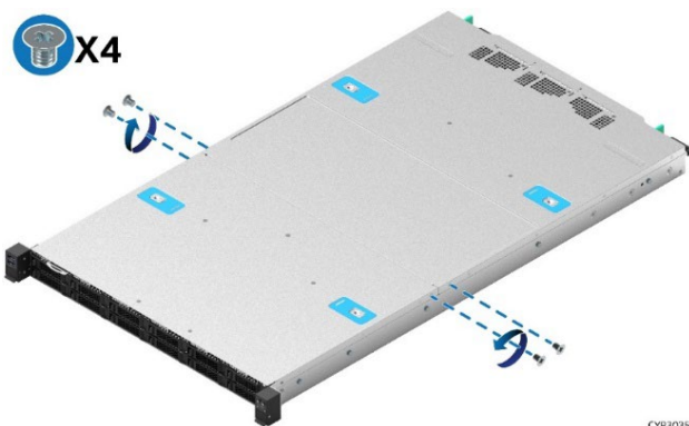
Figure 16. System Top Cover Shipping Screws
