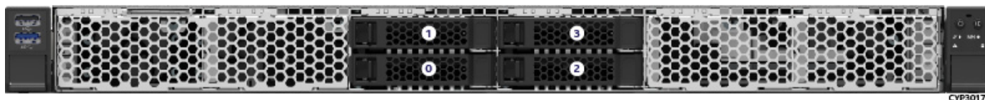
Figure 45. 4 x 2.5" Front Drive Bay Configuration – M50FCP1UR204
