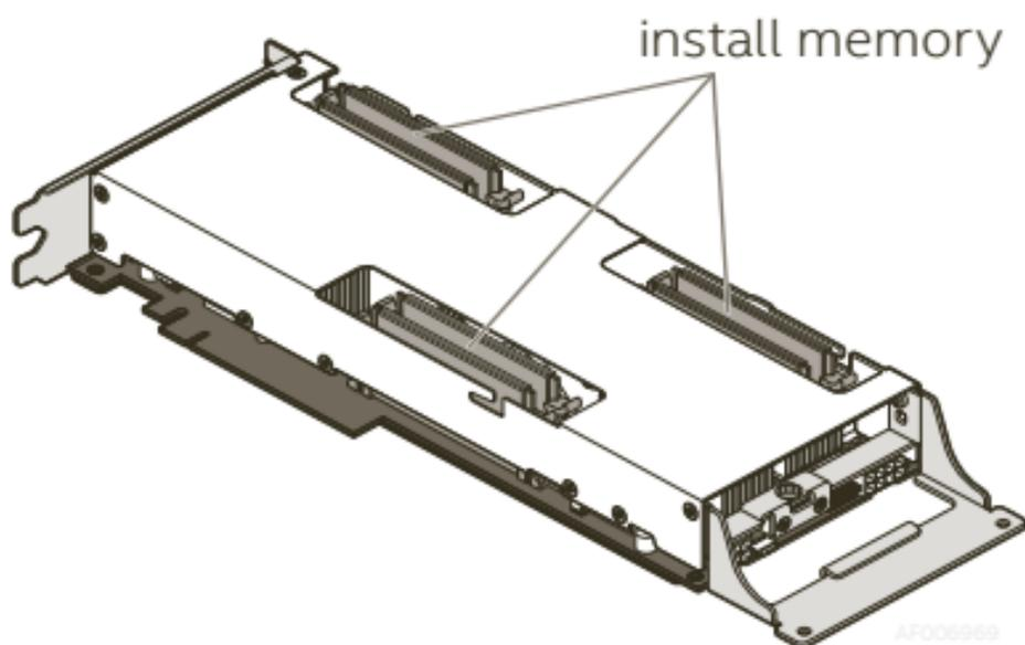
2. Insert each DDR4 ECC SODIMM vertically, ensuring that it is firmly latched in place (*Figure 2*).
