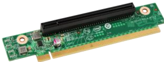
Figure 64. 1U one-slot PCIe* riser card (iPC – F1UL16RISER3)
