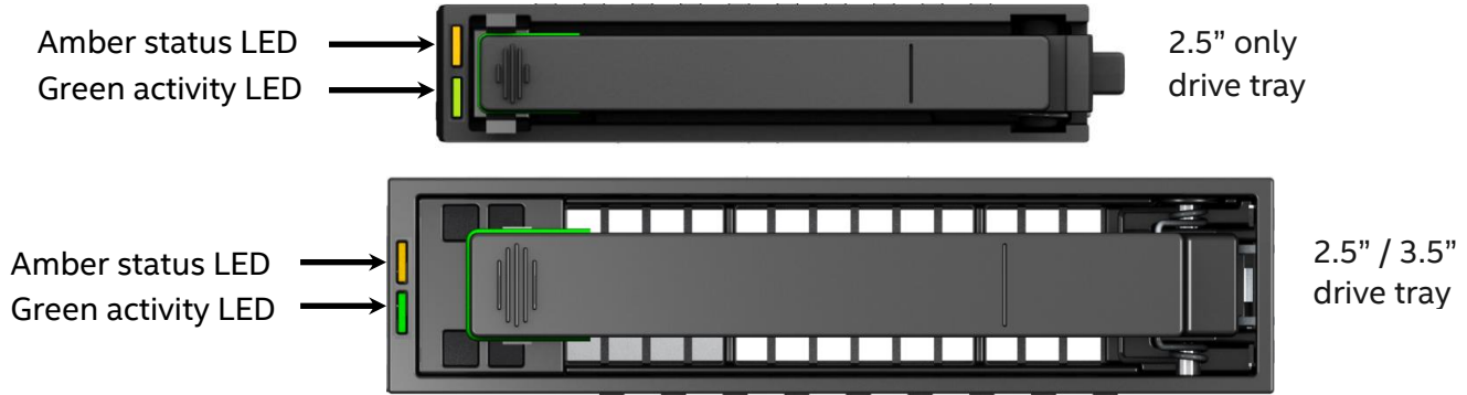
Figure 35. Drive tray LED identification
