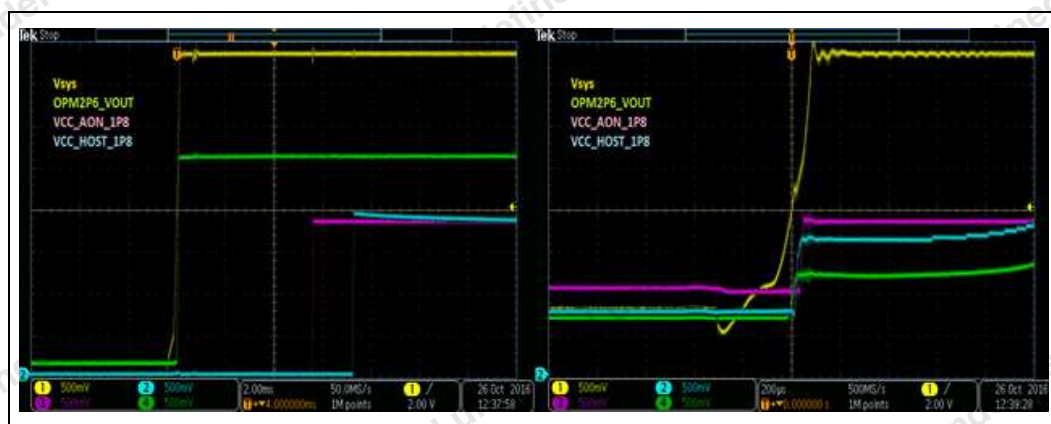
Figure 1. Intel® Quark™ SE Microcontroller C1000 Power Sequencing
