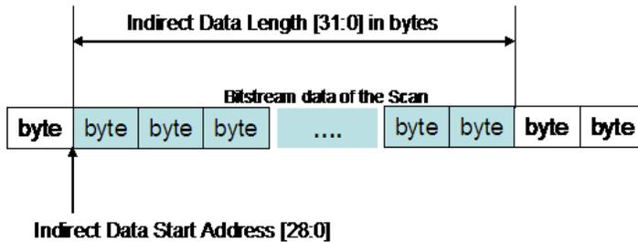
The indirect data length in MFD\_JPEG\_BSD\_OBJECT provides the length in bytes of the bitstream data for the Scan excluding Scan header. It includes the first byte of the first macroblock and the last byte of the last macroblock in the Scan. The Figure illustrates these parameters for a slice data.
