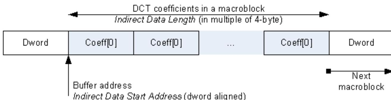
Each non-zero coefficient in the indirect data buffer is contained in a doubleword-size data structure consisting of the coefficient index, end of block (EOB) flag and the fixed-point coefficient value in 2's complement form. As shown in Structure of a transform-domain residue unit, *index* is the row major 'raster' index of the coefficient **within a transform block** (please note that it is not converted to 8x8 block basis). A coefficient is a 16-bit value in 2's complement.
