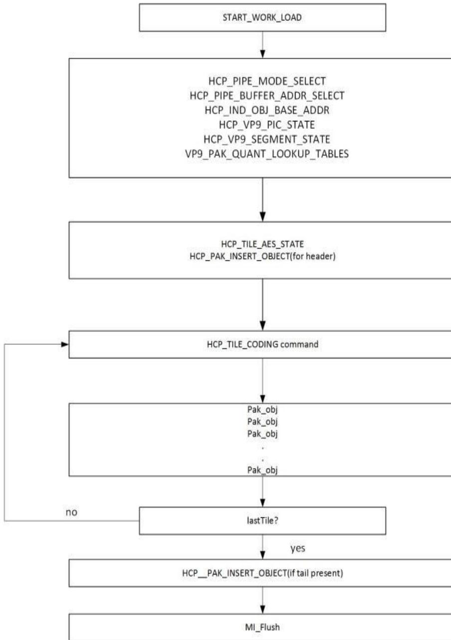
**VP9 encode command sequence for Single Pipe mode**
