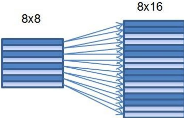
VertDownSamplingEnb is used to convert an input chroma422 to an output chroma420 in the surface format NV12. To enable this flag, the input should be interleaved Scan, InputFormatYUV should be set to YUV422H\_2Y or YUV422H\_4Y, and OutputFormatYUV should be set to NV12. Combined with AvgDownSampling flag, the following table and figures show the down-sampling methods.
