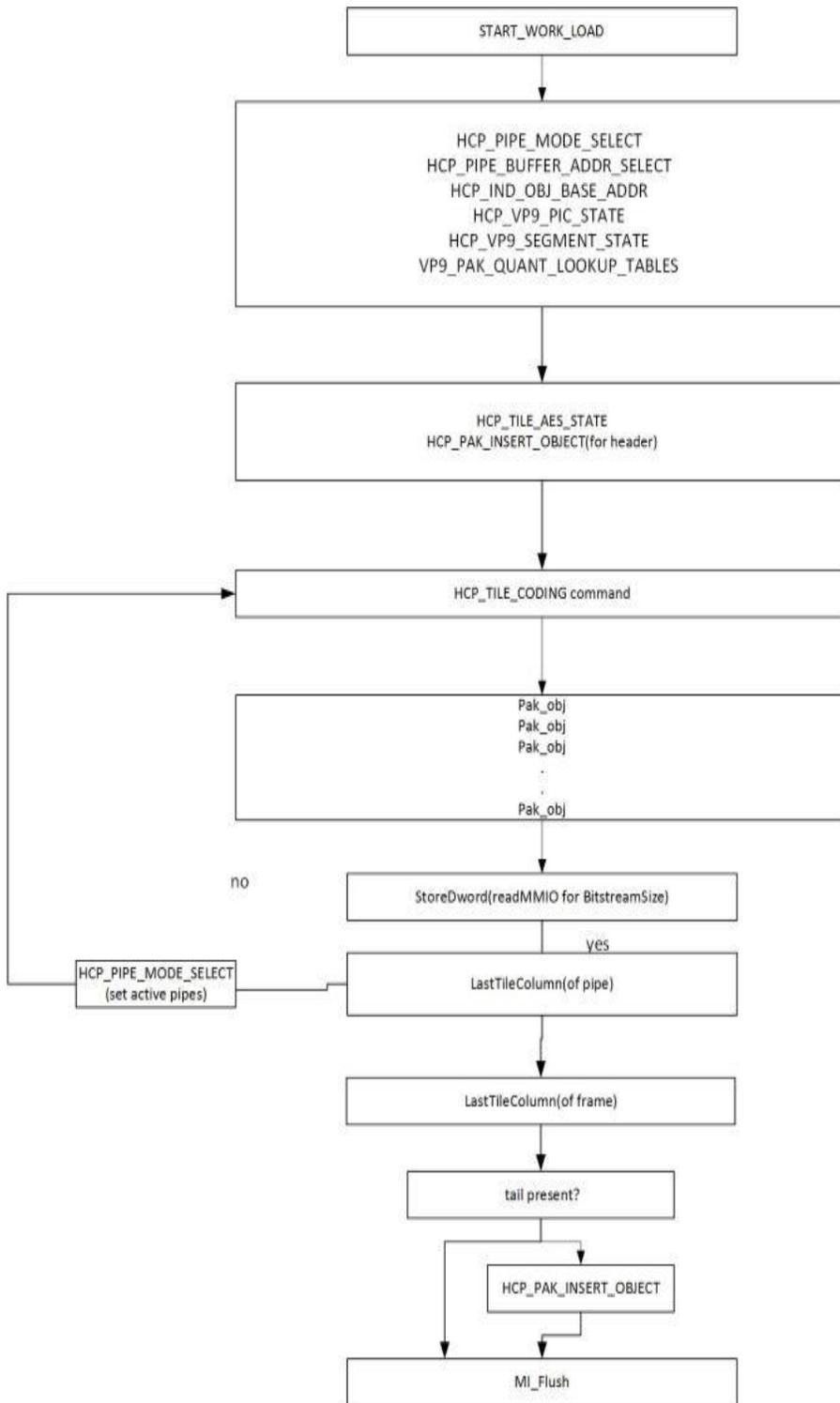
VP9 encode command sequence in Multiple Pipes mode
